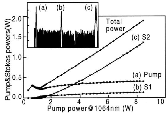
Fig. 2. Output powers of the residual pump, the first Stokes, and the second Stokes lights with change of input pump power and output spectrum at 1.36 W second Stokes power in inset.
