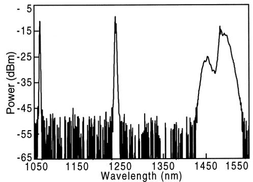
Fig. 4. Spectral continuum centered at 1484 nm generated by connecting the 1484 nm output to 500 m single-mode fiber.
