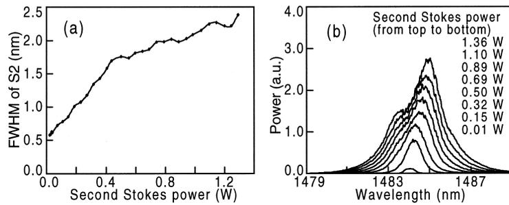
Fig. 3. (a) Spectral full-width at half maximum and (b) output spectrum of the second Stokes light at 1484 nm from the cascaded Raman fiber laser.
