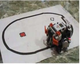
UEC students and UESTC students can collaborate to assemble Lego Robot with the ability to carry out omnidirectional movement, obstacle dodging and line patrol walking.
